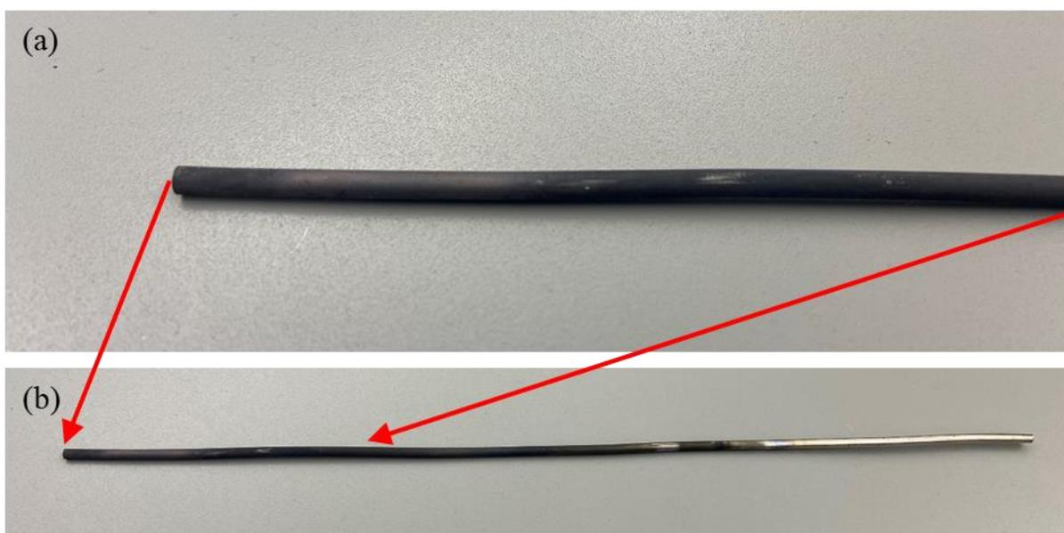
**Figure 16.** (a) Close up of black deposits observed on stainless steel rod used to hold catalyst in place. (b) Full length of stainless steel rod showing distinct line where the black deposit stops corresponding to the location where joule heating ends
