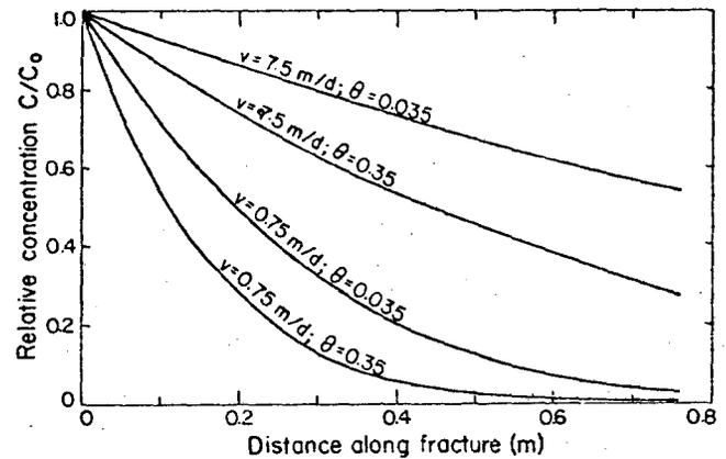
Fig. 7. Concentration profiles in the fracture at 0.2 day for various fracture velocities and matrix porosities. Matrix diffusion coefficient is assumed to be  $1 \times 10^{-6}$  cm<sup>2</sup>/s.
