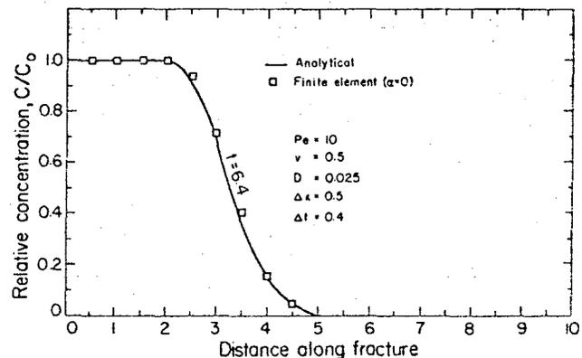
Fig. 2. Concentration profiles at  $t = 6.4$  comparing analytic and numeric solutions for  $Pe = 10$  in the fracture.
