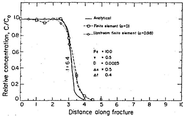
Fig. 3. Concentration profiles at  $t = 6.4$  comparing analytic, numeric, and upstream FE solutions.
