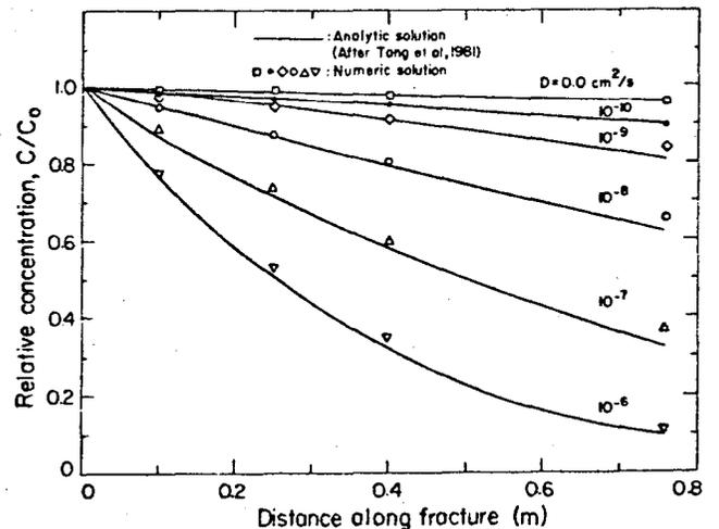
Fig. 5. Comparison between analytic solution of *Tang et al.* [1981] and numeric solution at 4 days.
