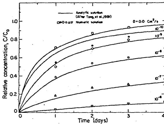
Fig. 6. Comparison between analytic solution of Tang *et al.* [1981] and numeric solution for breakthrough curves for fracture at 0.76 m from the source.
