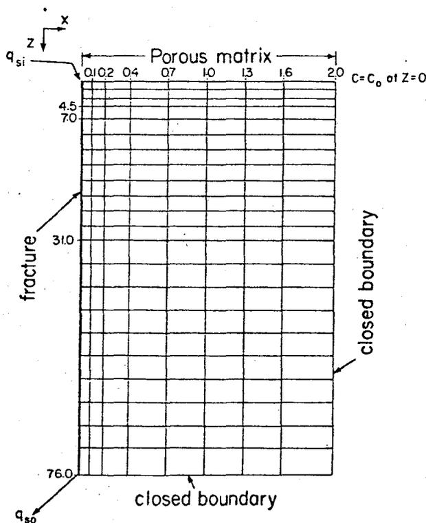
Fig. 4. Schematic diagram of the observation segment of the modeled region for two-dimensional solute transport (actual mesh extends to 234 cm). Dimensions are in centimeters.
