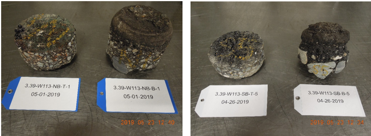
Figure 4.10: Examples of cores extracted from the newly placed RHMA-G.
