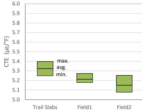
Figure 5.4: Concrete CTE (at age 42 days).
