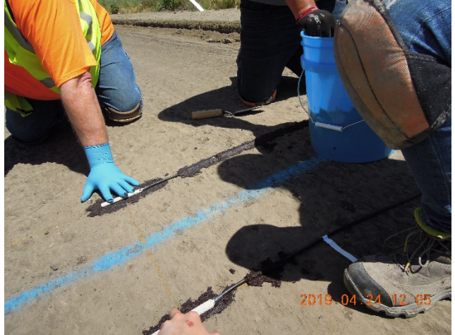
Strain gauges placed on SA bed (to prevent the milled surface from punching through the gauge during the RHMA-G compaction)
