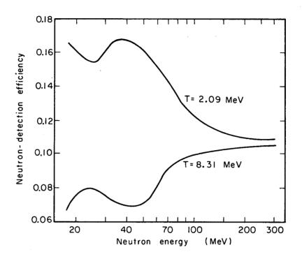
Fig. 12. Neutron-detection efficiency for a counter 10.16 cm thick with a fractional resolution τ of 0.15 and at detection thresholds T of 2.09 and 8.31 MeV.
