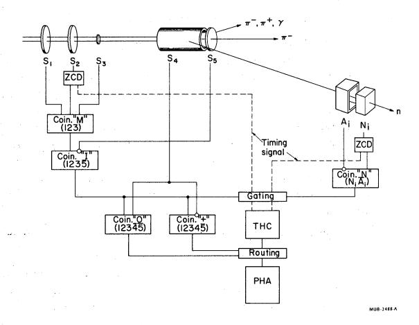
Fig. 9. Simplified electronic block diagram. Four neutron detectors  $(N_i \text{ and } A_i)$  were used in the experiment.
