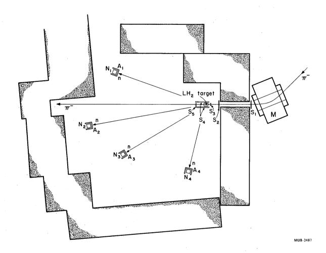
Fig. 6. Plan view of the experimental area showing target and counter arrangement.
