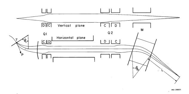
Fig. 2. Beam-optics diagram. C = convergent quadrupole element D = divergent quadrupole element T = internal Be target P = internal proton beam  $\theta = 67 \text{ deg}$   $\theta = 45 \text{ deg}$  L = 88.5 in
