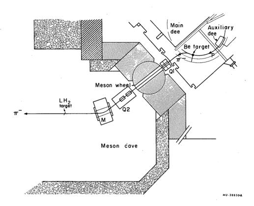
Fig. 1. Plan view of the meson cave in the 184-inch cyclotron showing the magnetic system for the pion beam. Detail of the target area is shown in Fig. 6.
