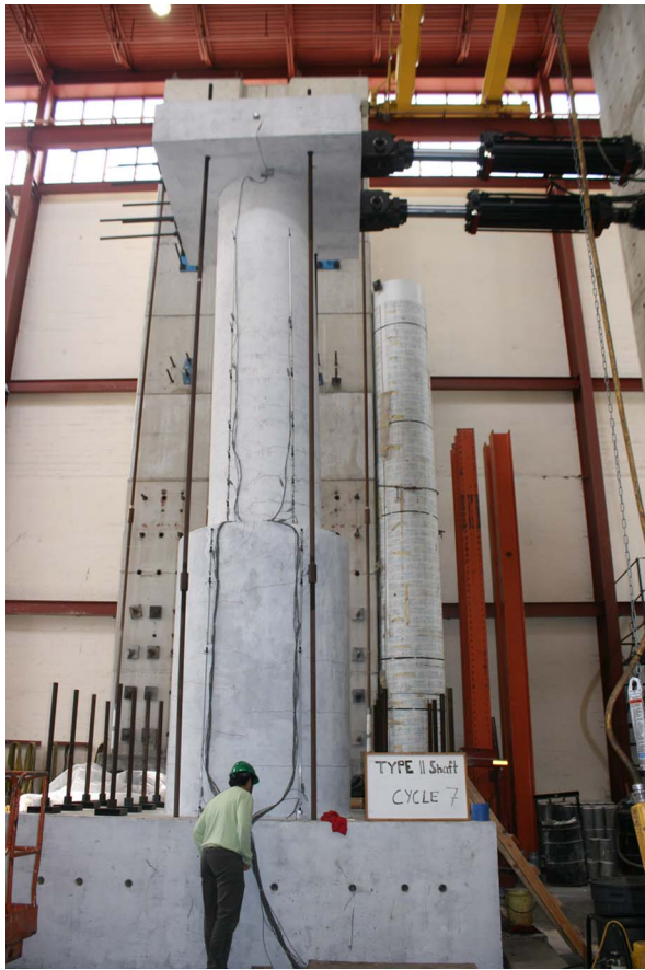
Fig. 1. Column-pile test specimen (reprinted from Murcia-Delso et al. 2016, © ASCE)
