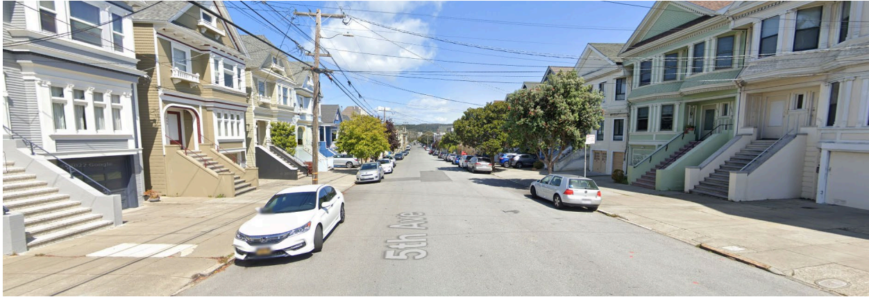
Figure 5.4. Large setbacks in many areas of San Francisco are expansive areas of concrete. These setbacks in the Inner Richmond neighborhood are about 8 meters from the curb to building façades, not including stairs. The streetscape is about 27 meters wide from building to building. (Image source: Google Street View)
