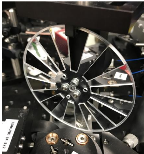
Figure 12. Reflective optical chopper wheel with 10 slots
