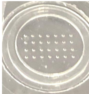
Fig.4.3. The PDMS stencil with 250 \mu\text{m} circular patterns.
