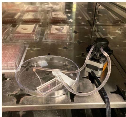
Fig.3.5. The human brain organoid shear stress controlled culture platform
