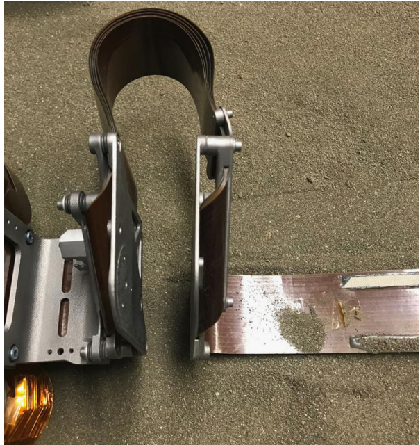
Fig. 31 Opening the Load Shunt Assembly (LSA) on the tether. The LSA mechanically decouples the seismometer from thermoelastic expansion and contraction of the tether
