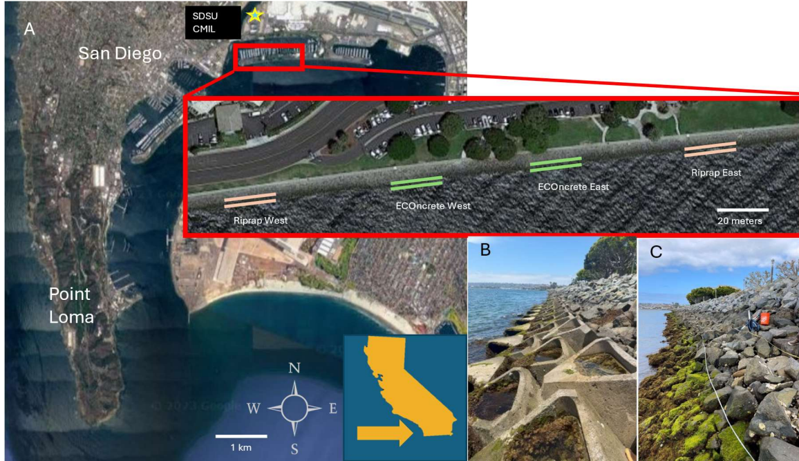
Figure 1: A) Map of Harbor Island, San Diego, CA (32.724435, -117.206360); B) COASTALOCK installation; C) traditional riprap.
