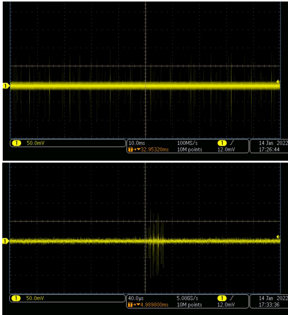
Figure 2.6: Sample measurement of the X-ray pulse at chopper setting 2000. (Top) Full view of the measurement window. (Bottom) Zoom in view of a single X-ray pulse.
