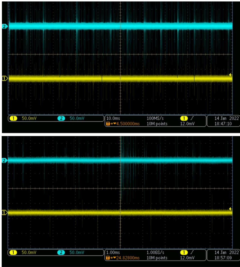
Figure 2.7: Sample measurement of the GOS:Eu 3+ optical pulse at chopper setting 2000. (Top) Full view of the measurement window. (Bottom) Zoom in view of a single optical pulse. The yellow signal corresponds to the X-ray pulses while the blue signal corresponds to the optical pulses.
