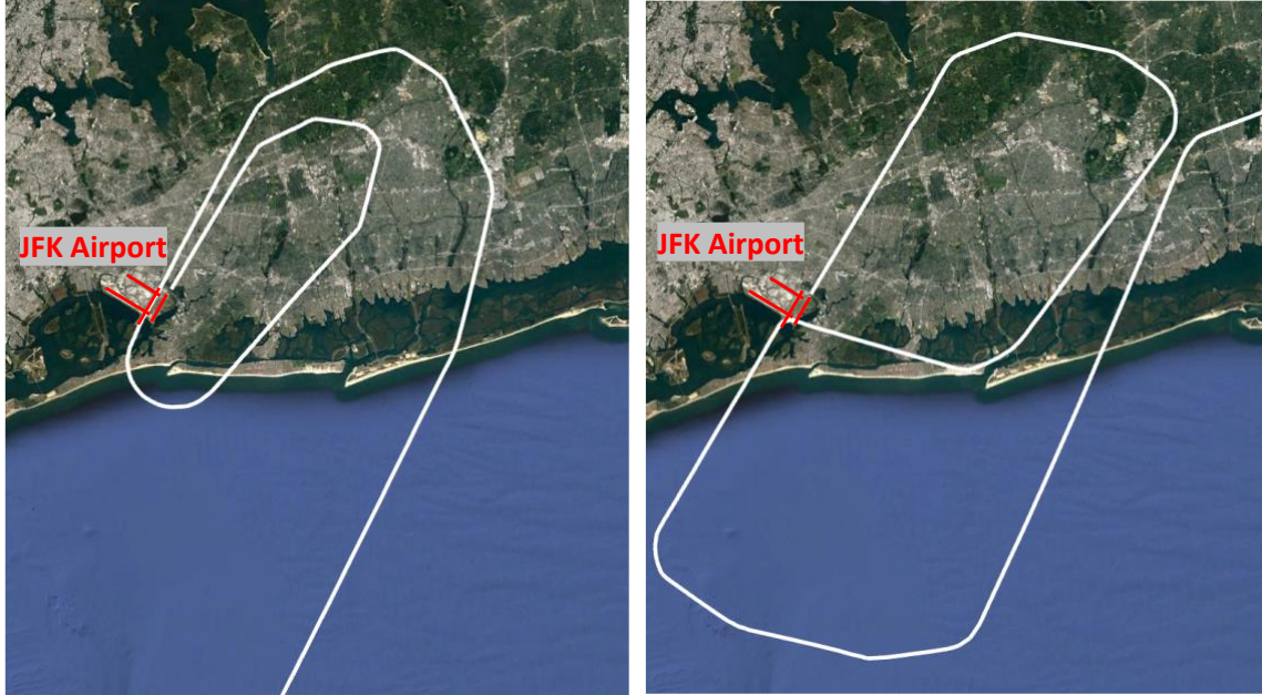
Figure 10. Exemplified go-around flight trajectories.
