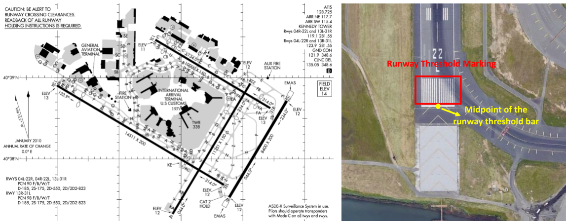
Figure 9. JFK airport chart (left) and the runway threshold marking (right).
