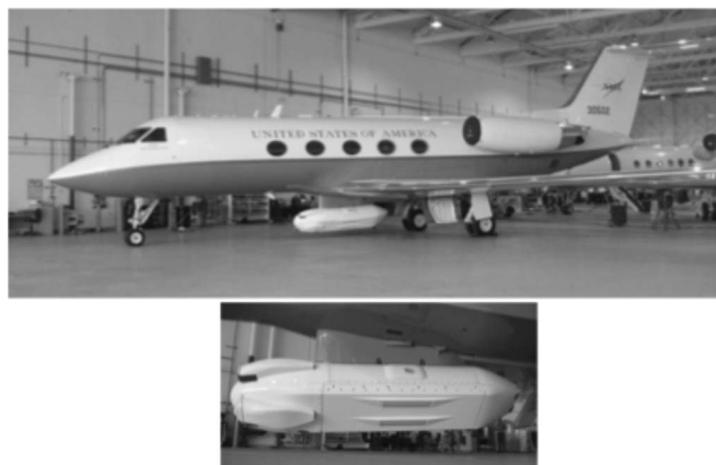
Fig. 3. Photograph of NASA G-III with pod configured for Ka-band interferometry. Lower inset shows a close-up with details of the two antennas.
