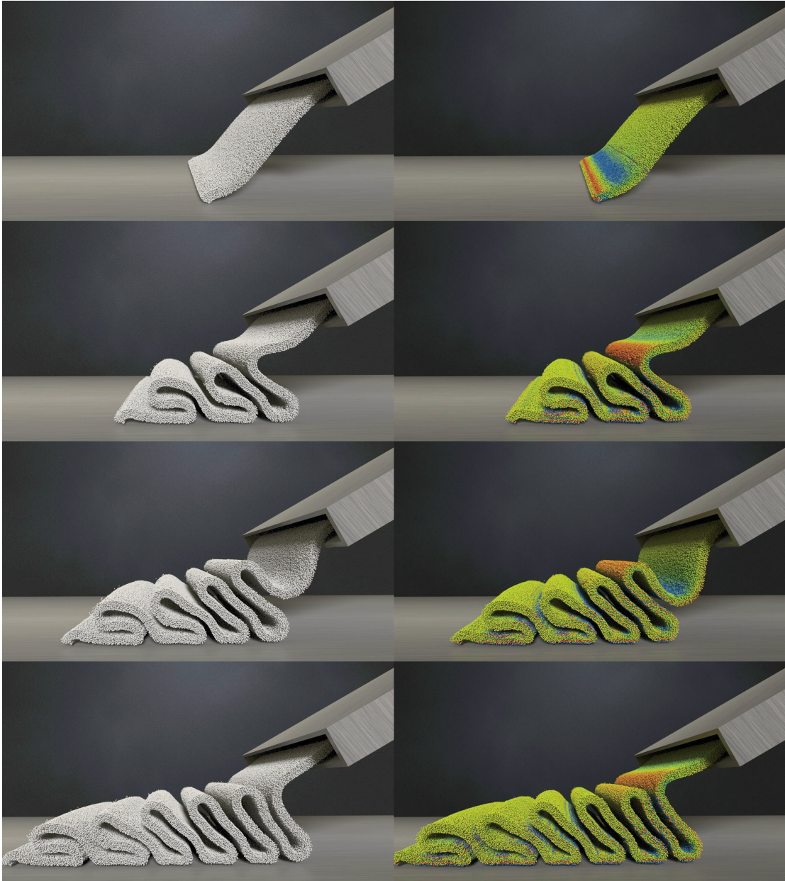
Figure 5.7: Particle rendering of Viennetta ice cream. Colored particles on the right correspond to the determinant of the left elastic Cauchy-Green strain on a particle: red particles have determinant greater than 1, blue particles have determinant less than 1.
