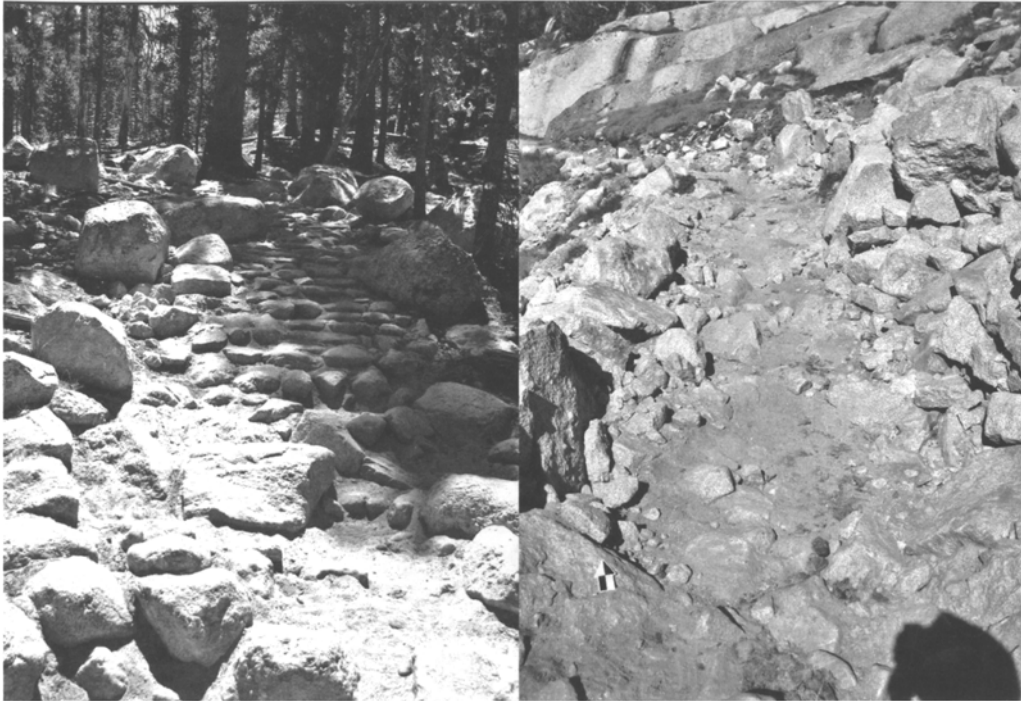
FIGURE 9. Examples of trail surfaces with differing localized topographies, cobble counts, and interstitial matrices ( left : sand, right : decomposed granite). (Photo by author, 2011.)
