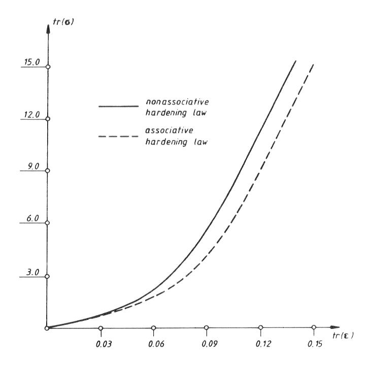
Fig.7 - Predicted hydrostatic behavior for McCormick Ranch Sand
