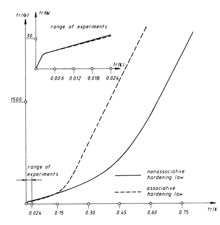
Fig.6 - Predicted hydrostatic behavior for the Colorado Conrete Data
