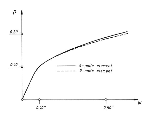
Fig.5 - Load-displacement curves for the plane strain, flexible footing problem
