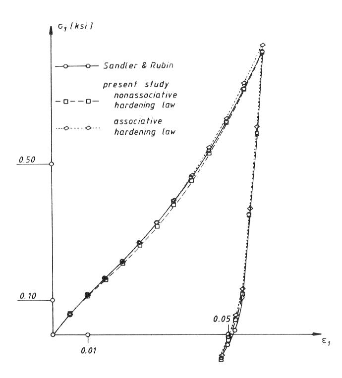
Fig.4 - Uniaxial strain test for McCormick Ranch Sand
