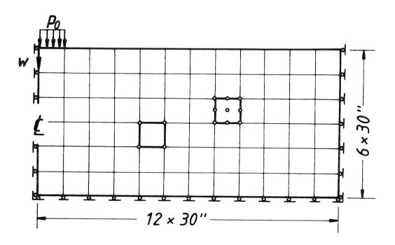
Fig.3 - plane strain, flexible footing problem
