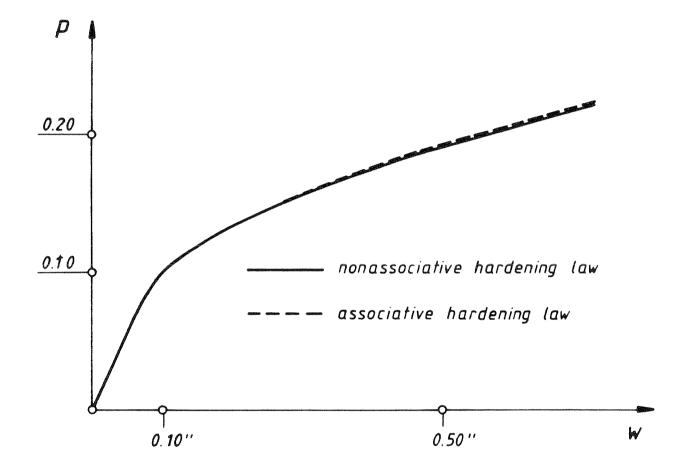
Fig.8 - Load-displacement curves for the two hardening laws (4-node element)
