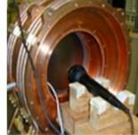
Figure 4. Pendulum and Be window in 805 MHz cavity (Left). Microphone measures acoustic response. (Right).
