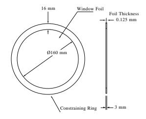
Figure 1: Layout of Beryllium test window [units: mm]
