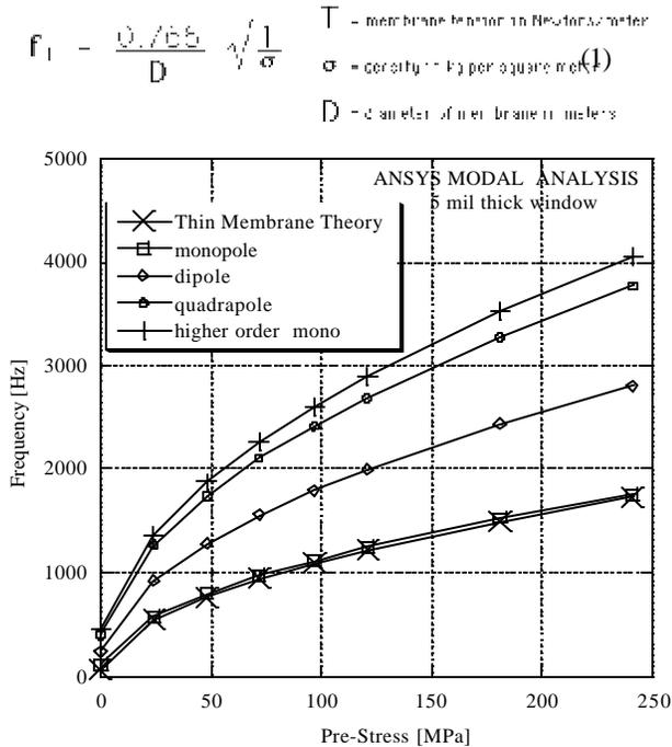
Figure 5: Theoretical and ANSYS FEA predicted frequency response versus Pre-Stress for 5 mil foil
