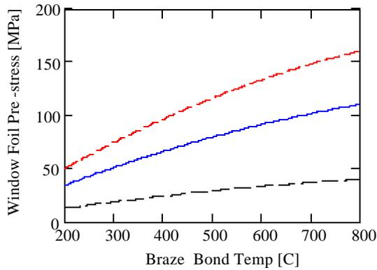
Figure 2: Theoretical pre-stress in a 16 cm window as a function of braze temperature. Cases shown for a Delta CTE of 8% (top), baseline 5% (middle) and 2% (bottom).
