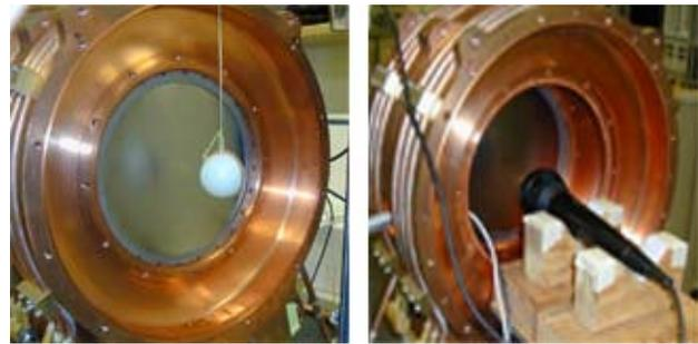
Figure 4. Pendulum and Be window in 805 MHz cavity (Left). Microphone measures acoustic response. (Right).
