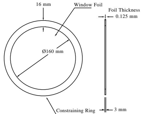
Figure 1: Layout of Beryllium test window
