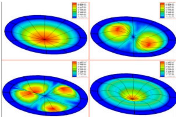
Figure 6: Pro/Mechanica 3D FEA modal analysis. Mode shapes for a 16 cm diameter, 0.127 mm thick window. Prestress: 50 MPa, (left to right, starting top) 822Hz, 1319 Hz, 1781 Hz, 1918 Hz.
