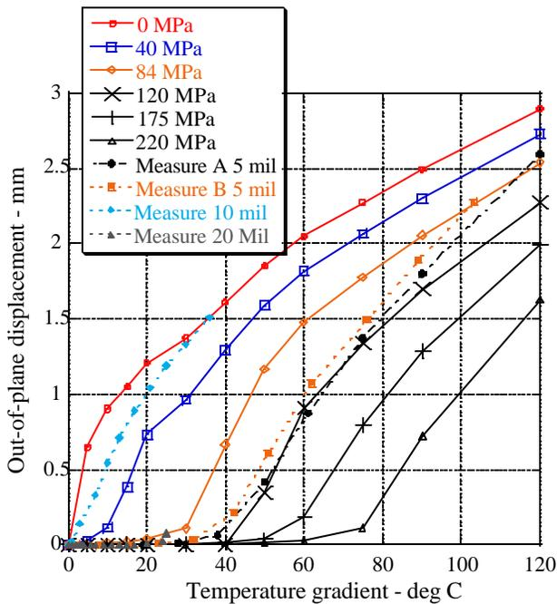
Figure 3: Thermal gradient and out-of-plane displacement. Experimental and ANSYS data.
