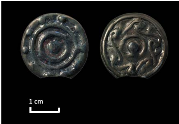
Figure 5.5: Cast pendant (ETD 98/21) from Boğazköy. This broken pendant is produced with an exceptionally high arsenic content (26.9% As) and low traces of other elements. This alloy is distinctly silvery in color.
