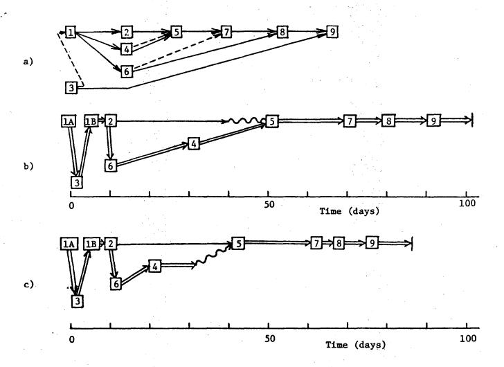
Fig. 1 Task sequencing of a typical graduate research program: a) arrow diagram, b) critical path for a normal program rate, c) critical path for an accelerated rate.
