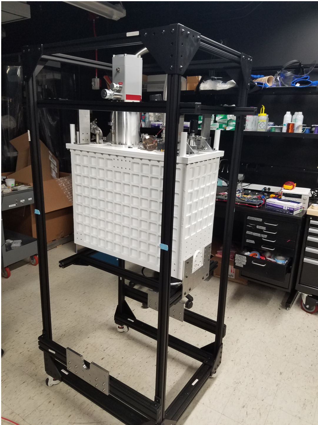
Figure 2.6: The PICTURE-C cryostat mounted on its lab frame with the pulse tube installed. The cryostat is upside down compared to the flight configuration.
