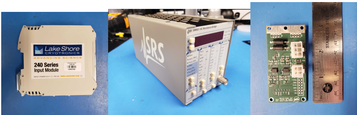
Figure 2.21: Left: A Lakeshore 240-2P will monitor the nitrogen and helium stage temperatures. Center: A SRS SIM921 AC resistance bridge will measure the temperature of the device stage, while an SRS SIM960 (not pictured, but looks similar to the 921) provides PI feedback to the ADR power supply. Right: The PIPER power supply will source current for cycling and regulating the ADR.
