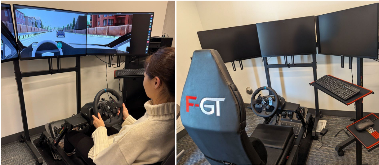
Figure 4: The Driving Simulator Setup, Consisting of the Physical Steering Wheel, Cockpit, Seat, and Pedals, the Triple Monitor Configuration, and the Virtual Driving Environment OpenCDA.
