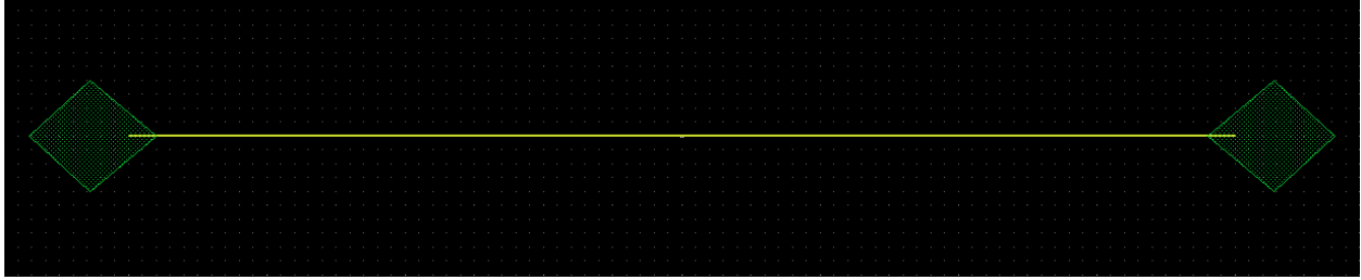
Figure 3.37: Pattern for the nanowire including anchors at the ends.
