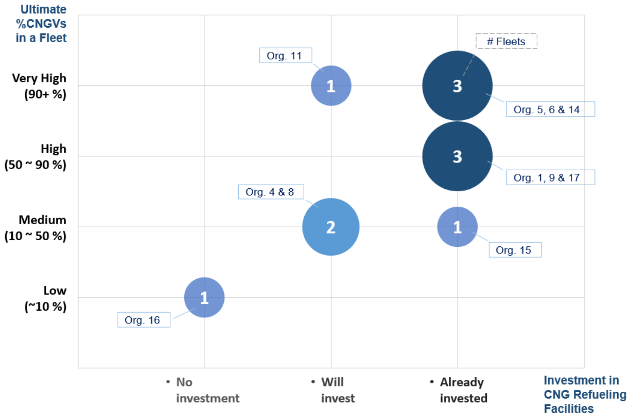
Figure 4-19. A Rough Trend between Investment in Refueling Facilities and Penetration Rates of CNGVs: Only with the Satisfactory Cases
