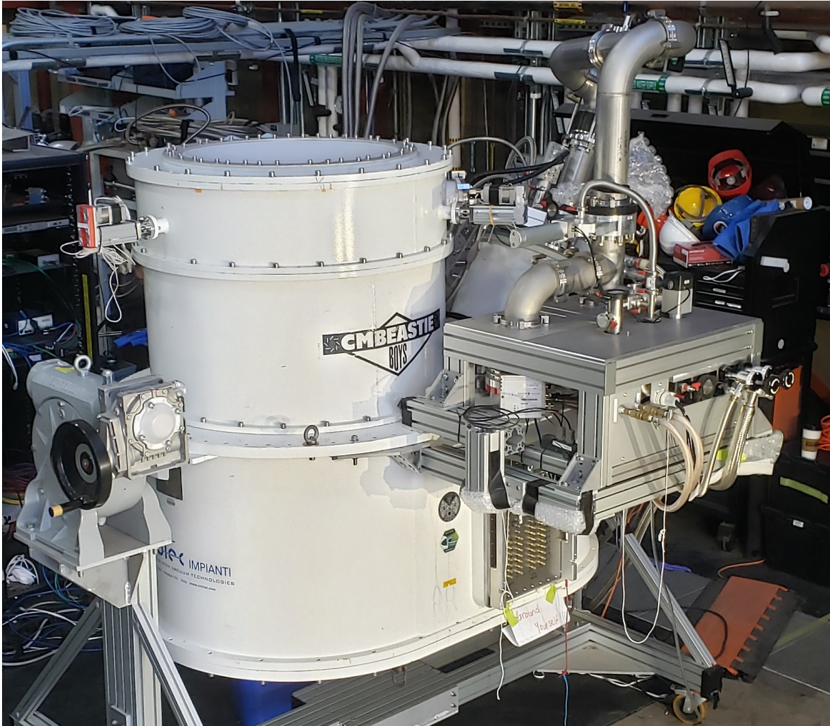
Figure 4.4. The fully assembled SAT-MF1 in the UCSD laboratory space. The rack mounted to the side houses the turbo-molecular pumps for the DR circuit and is attached to the receiver with a mounting jig for testing in the lab.
