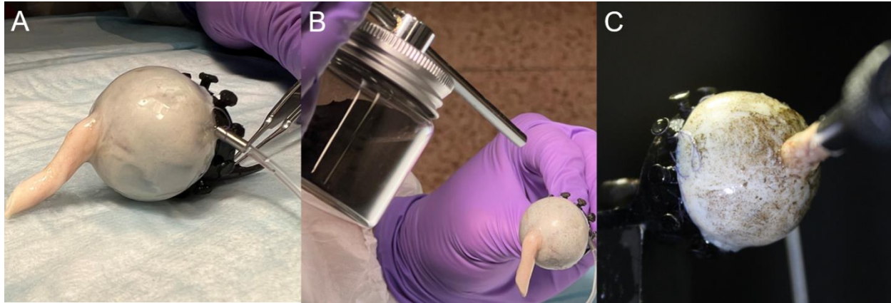
Figure 26. Sample preparation. (A) Globe was sutured to fixation ring, and infusion cannula inserted in anterior sclera. (B) Speckles of cast iron dust were randomly applied to the surface by using a pneumatic applicator. (C) Speckle pattern on the sclera.
