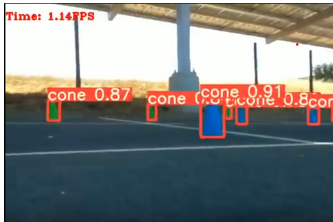
Figure 7.2: Cone detection using the YOLOv5 object detection mode. The images are taken from the AGV. The model returns the bounding box coordinates and confidence level of the detection. The inference frame rate is displayed at the upper left corner of the image. This model was run on the SBC—we have successfully deployed the EfficientDet model to the TPU with significantly faster inference times.
