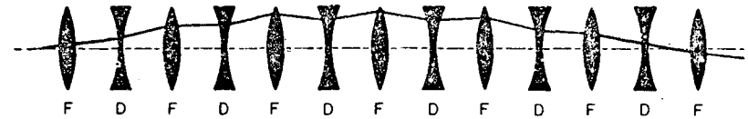
FIG. 1. Optical analogue of alternating-gradient focusing, showing a ray traversing a periodic sequence of focusing ( F ) and defocusing ( D ) lenses.
