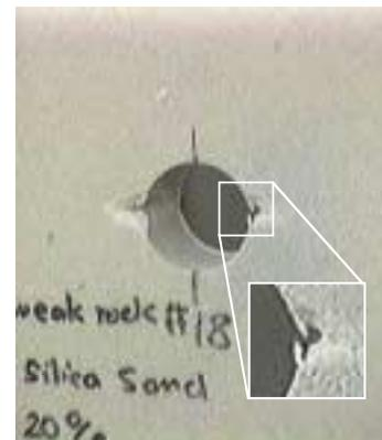
(c)  $S=10\%$ . Extensile fractures in borehole wall were observed.
