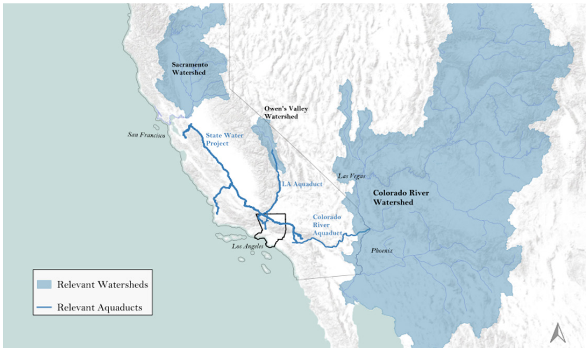
Geographic map of the western United States showing Los Angeles's water import aqueducts and their respective watersheds
