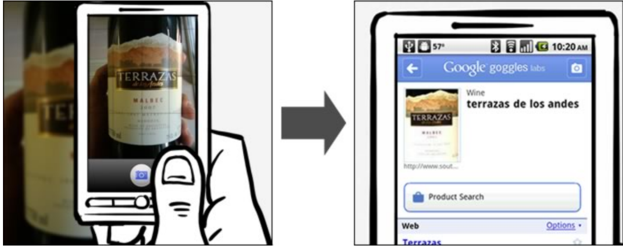
Figure 4.4: A photo taken by a smartphone can be uploaded to the Google object recognition engine where it is analyzed, and results such as a list of relevant websites are returned to the user. We use a variant of this system where results determine object identity, pose, and appropriate grasp strategies.
