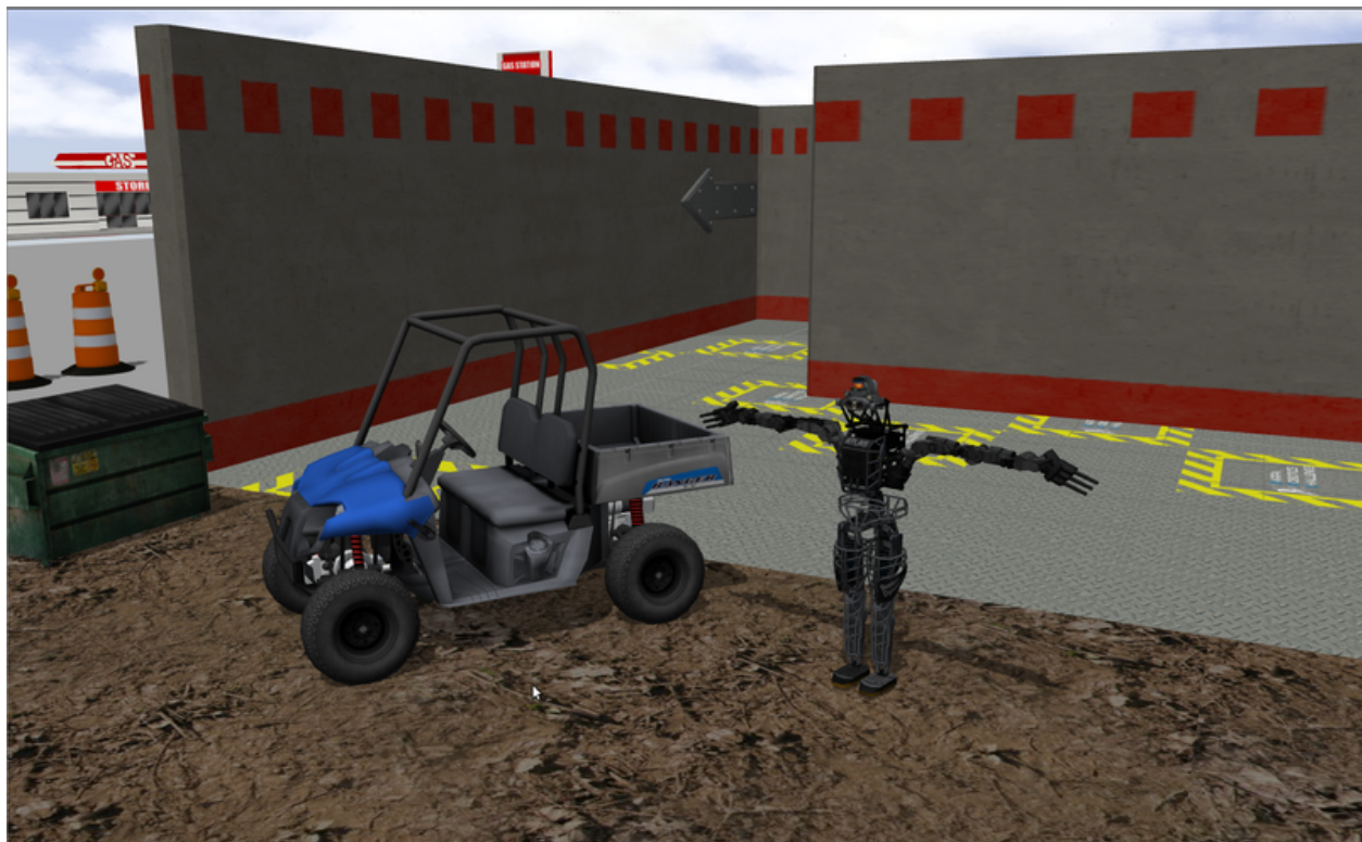
Figure 2.12: The DARPA Robotics Challenge (DRC) used CloudSim, an open-source Cloud-based simulation platform for testing the performance of the Atlas humanoid robot (shown) on a variety of disaster response tasks [72, 40]. The Cloud permits running interactive, real-time simulation tasks in parallel for purposes such as predicting and evaluating performance, validating design decisions, optimizing designs, and training users. This competition also resulted in enabling sharing of robotics research efforts. (Image reproduced with permission).
