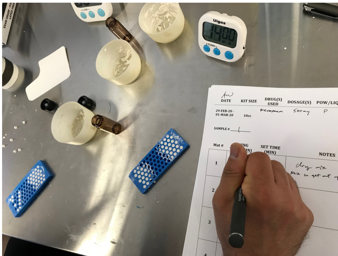
Figure 1. Photograph of 4.8 mm bead mat. The antimicrobial-loaded \text{CaSO}_4 paste is shown after spreading the paste into the molds. Once applied, the bead mats were left on the countertop to set, in order to imitate operating room procedure. Time measurements were recorded to establish a set time for each formulation.
