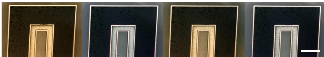
Figure 4.8. pH changes detected optically in NaCl with pH indicator solution. The palladium contact (black) cycled between -1\text{V} and +0.3\text{V} vs an AgCl pellet electrode for 1 minute at each voltage. The solution switched between an initial neutral solution (yellow) at t=0\text{s} (left), to basic pH (blue) at t=60\text{s} after 1 minute of -1\text{V} on the Pd (second from left). The cycle was repeated neutral conditions at t=120\text{s} after +0.3\text{V} on the Pd, and basic conditions at t=180\text{s} . Scale = 0.4\text{mm} .
