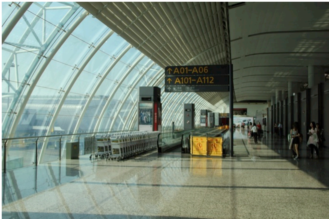
Figure 5. From the moving walkway, the altitude angle to the top of the window is approximately 60°. Since the width of the window is very large, we have a f_{svv} value of about 1/3.
