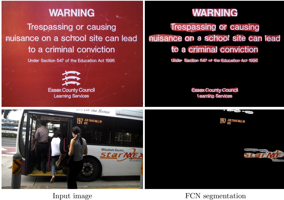
Figure 3.2: FCN is in general unable to separate individual words.
