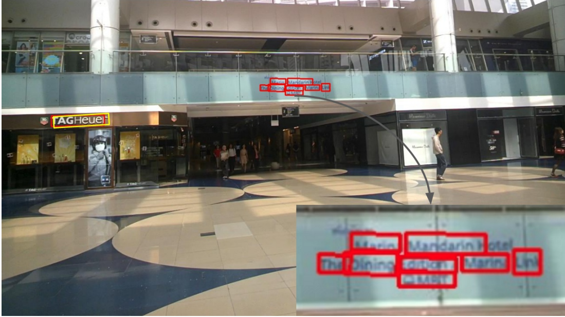
Figure 3.3: By cascading segmentation (TextSegNet) with detection (WordDetNet), our algorithm can detect both large and small words. If only WordDetNet is used, as trained on whole images, detection will fail in the case of too small words. Detected words by TextSegNet + WordDetNet are shown by red rectangles, the result of WordDetNet only are shown by yellow rectangles.
