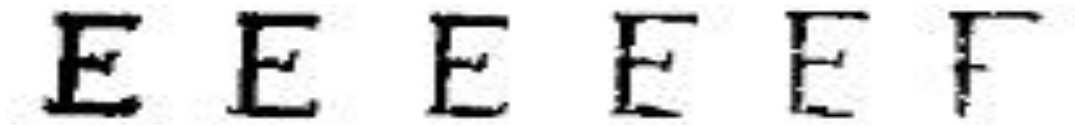
Figure 2.3: MSERs within a cluster centered at the red rectangle (only a few shown). The MSERs are ordered in decreasing value of fullness . The MSER to the left is chosen as the cluster representative
