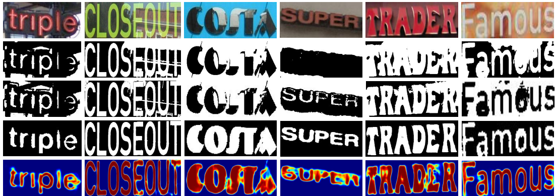
Figure 4.5: In this figure we compare the result of Otsu binarization algorithm [59], Zhou’s text segmentation algorithm [103] and our method with several challenging images. From top to bottom: input image, Otsu result, Zhou’s result, our result and our raw FCN output probability map.
