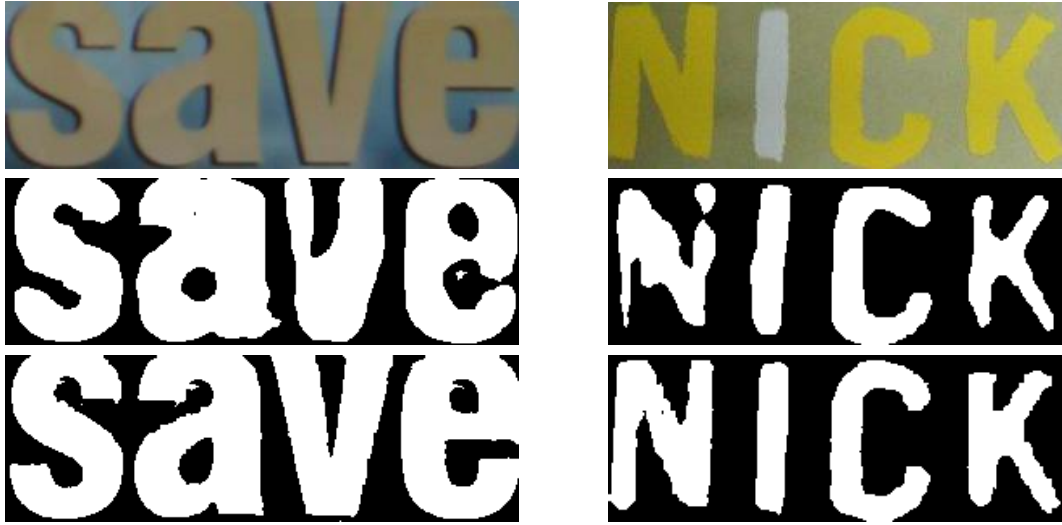
Figure 4.3: The first row is input images, second row is raw FCN predictions and last row contains final results with CRF refinement.
