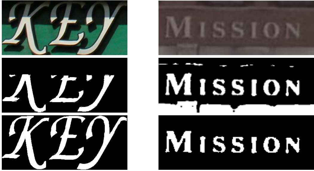
Figure 4.4: The first row is input images, second row is results without stroke width kernel and last row contains results with stroke width kernel. In left example the text color has large variance due to shadow and for right image the background contains regions with similar color as text region. In these cases use bilateral kernel alone becomes unreliable.
