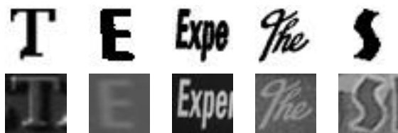
Figure 2.2: Some resized binary patches fed to CNN, together with their original grayscale counterpart. Note the presence of a trigram and of a four-gram.
