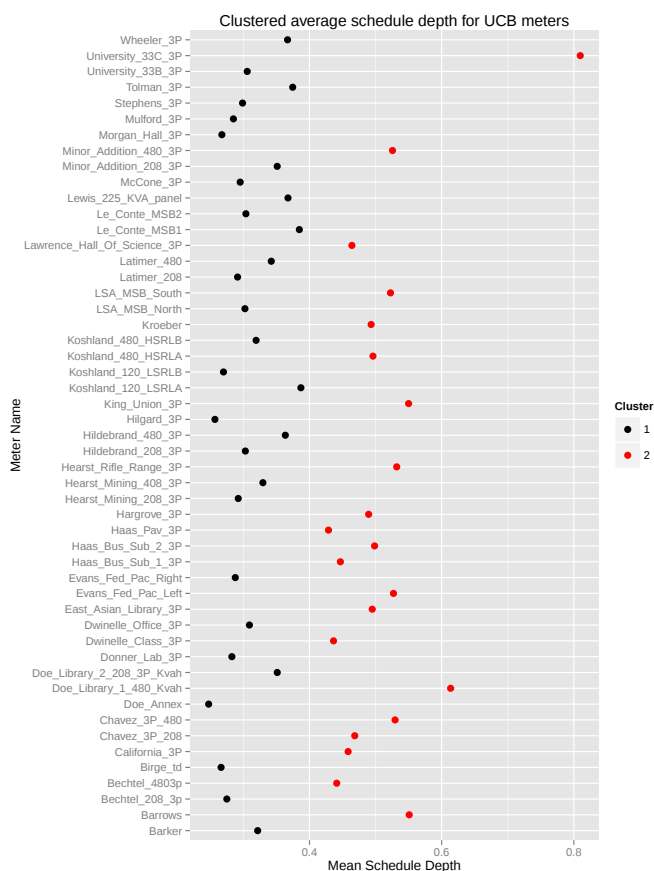
Figure 6.2: Mean schedule depth for meters in our data set. This group was divided into two cluster that represent two different operational modes, corresponding to the previous two peaks in fig. 6.1.
