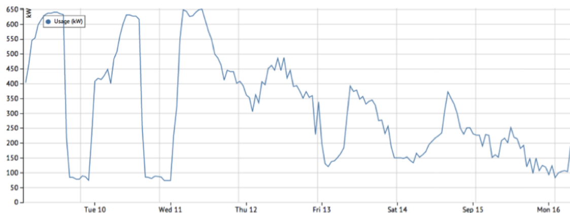
Figure 4.10: The algorithm picked up this point in the power usage of Building 2 that showed the building not shutting down correctly at night.
