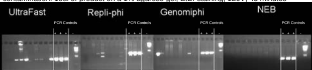
Figure 1b: 16S PCR products run on ~50ng of MDA DNA. Commercial kits show bacterial contamination. 1oul of product on a 1% agarose gel, EtBr staining, 120V, 45 minutes
