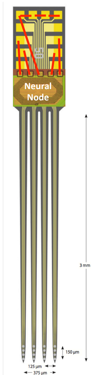
Figure 4.1: An implantable neural recording probe offered by NeuroNexus, the head of the probe is approximate 450\mu\text{m} wide. A die photo of the neural node is oriented in the approximate location for die attach and a potential bonding diagram is shown in red, allowing for 1 recording per shank. A large area reference electrode through the is created by stitch bonding multiple recording sites.
