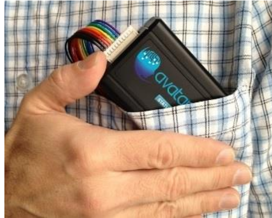
Figure 3.4: Pocket-sized Avatar EEG recorder
