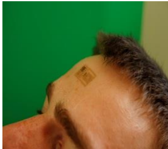
Figure 6.2: Futuristic wireless single-channel EEG based unobtrusive, seamless sleep monitoring device
