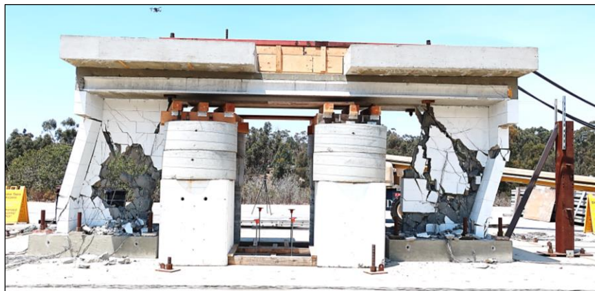
Figure 5-12. Damage in Specimen 1 after the quasi-static pull test
