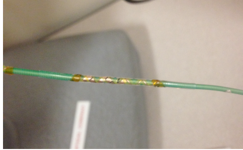
Figure 4: Manually cut out resonators wrapped around catheter with outer radii of 0.087". Copper layers do not touch and circuit was completed via silver epoxy.
