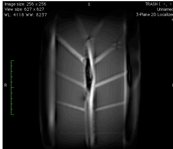
Figure 9: Poor visualization of the catheter and guidewire, without the resonator, in the abdominal phantom during timing test for experience and inexperienced user.
