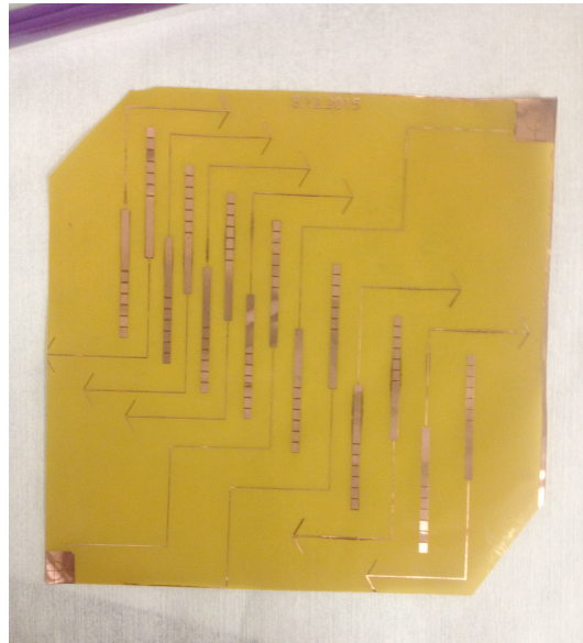
Figure 3: Completed resonators on the pyralux sheet. One leg from the apex is the capacitance section where the squares incrementally change the capacitance. The other leg is the inductance section.
