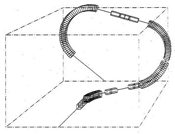
This was needed to fix the beam at a variable twist in a transport system. The flexibility and modularity of LATTICE allows additional complex types of constraints to be easily added to the source code, which must then be recompiled.
