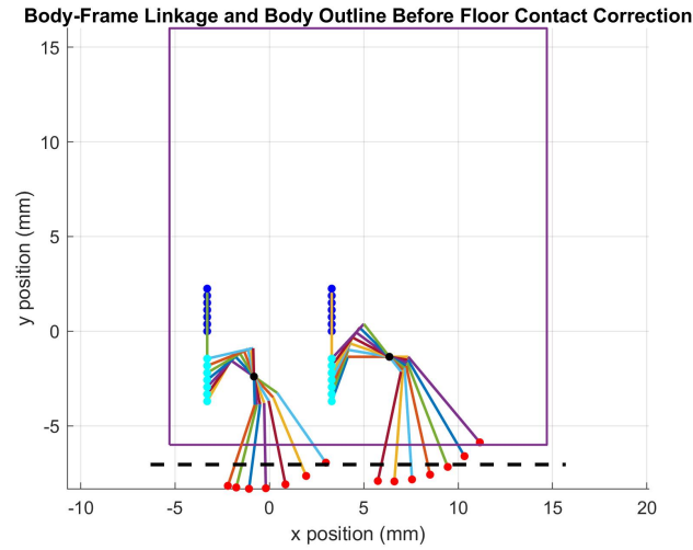
Figure 5.9: Body-frame linkage poses for the crab-inspired mechanism over the prescribed shuttle stroke. The linkage geometry is shown before transformation into the world frame, so the shuttle, input linkage, dual connector linkages, and vertical ground linkages retain their body-frame translational constraints. The rigid walking surface is included as a reference line, but contact correction has not yet been applied in this frame.
