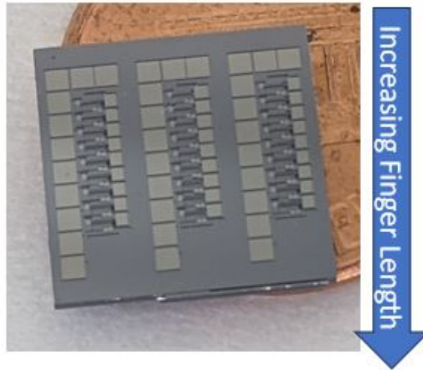
Figure 6.9: As-fabricated PIPO test chips shown before full separation from the break-away tabs. The array layout permits multiple GCA geometries to be inspected and tested from a single fabricated chip.
