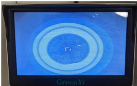
Figure A.6: Image of the backside etch process through the view port of the STS-2 tool showing the wafer on the chuck within the vacuum chamber as plasma is active (blue color).
