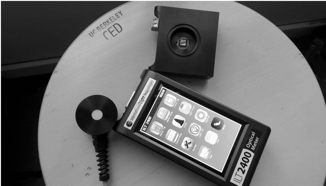
Figure 4: Photodiode-based handheld light meter and data logging device w/ optical filter engineered for EML.
