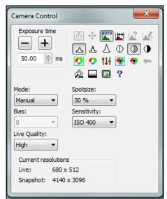
This panel adjusts exposure time, sharpness, contrast, and white / black balance. The Mode should usually be "Manual"
