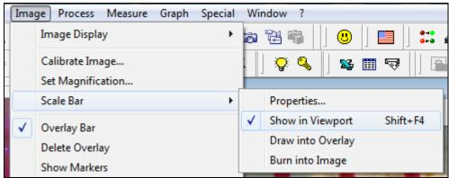
Click Image > Scale Bar > Properties. Select the attributes desired for Display, Format, and Size. The font size (under the "Size" Tab) recommendation is 48 as Microsuite likes multiples of 12 (Note: you will not be able to "see" your changes in the view screen, but Scale Bar Properties
