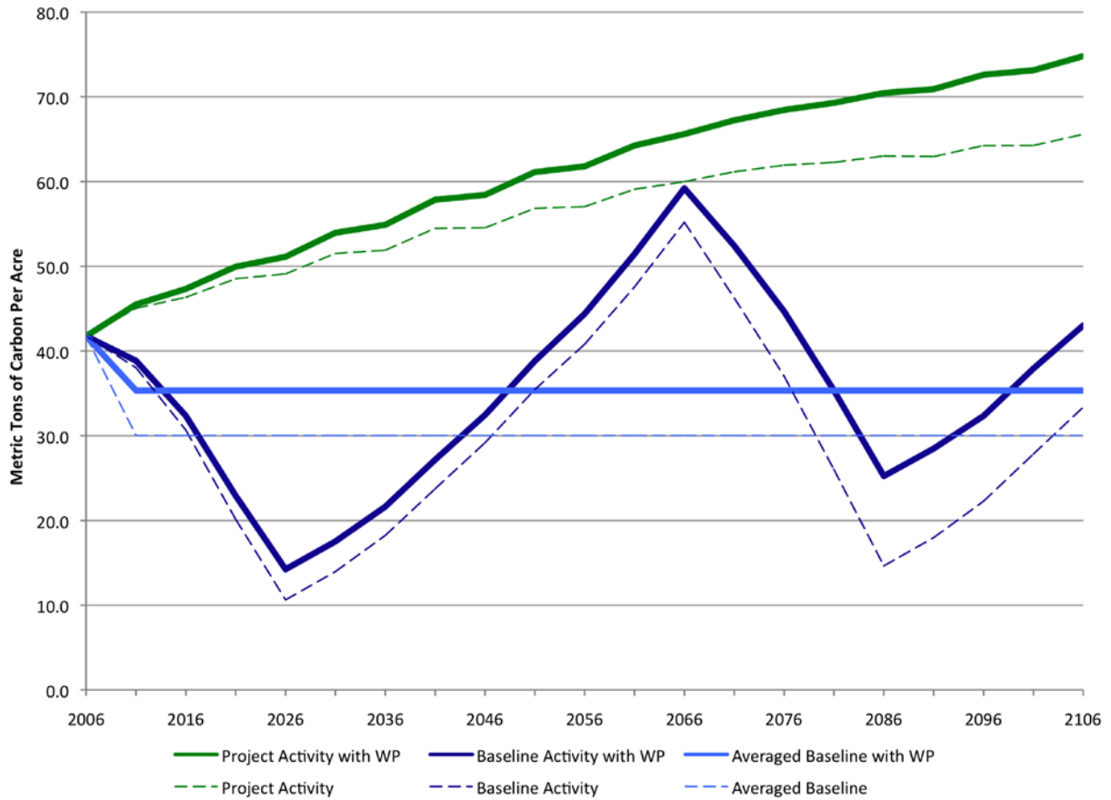
Figure A1. Baseline and project activity carbon stocks, both with and without wood products pool stocks, over the 100-year project lifetime on a per acre basis. The averaged baseline activity value is also shown. All scenarios have the same initial carbon stocks at the project start date in 2006. The averaged baseline curve begins at this same starting value, but achieves the average value by the end of the first 5-year reporting period by being reduced annually in equal increments.
