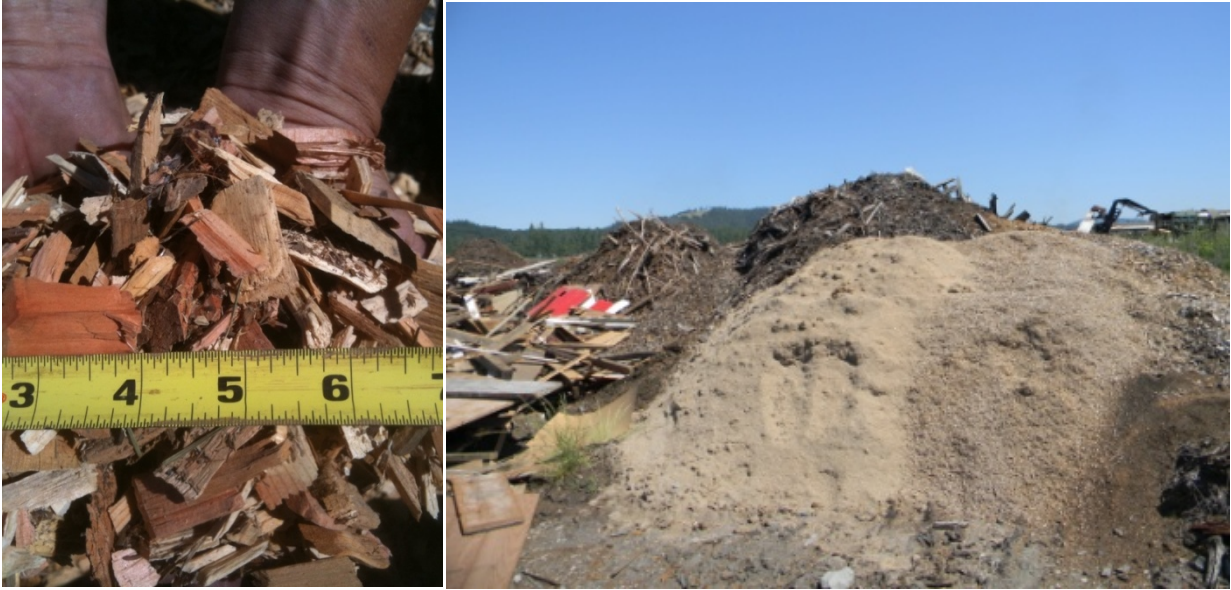
Figure 3. Wood waste used in the TSY-Peak biochar system. Left is the hog fuel used to power the gasifier. Right is the waste biomass currently left to rot in the log yard, which feeds the pyrolytic retort. Photo Credit: Matt Delaney (left) and Peter Weisberg (right)
