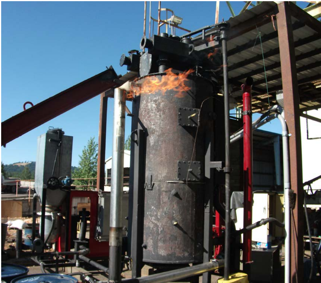
Figure 2. Fluidyne Gasifier (left background, metallic surface) and pyrolytic retort (right front, black paint) in the log-sorting yard of Thompson Timber/Starker Forest, Philomath OR.
