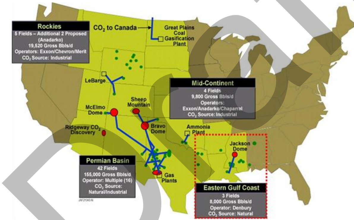
Figure 13. Map showing location of major CO 2 pipelines for EOR in the United States 84
