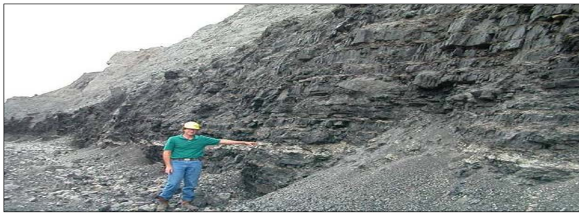
Figure 31 : 15-m thick Big Dirty Seam at the Centralia mine, with white bentonite tuff parting.
