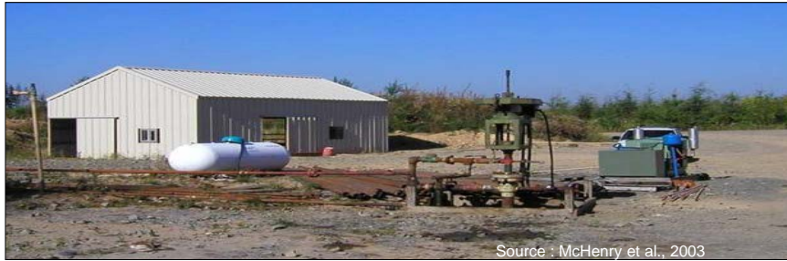
Figure 12 : Coalbed methane completed wellhead, El Paso Inc. Carbonado pilot area.
