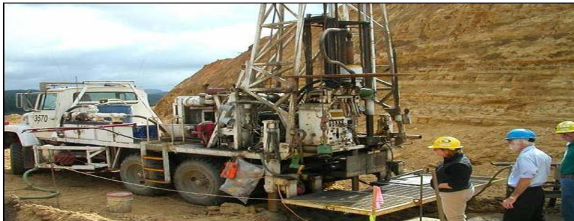
Figure 4 : Wireline coring rig (800-ft max) targeting the Big Dirty Seam at the Centralia mine.
