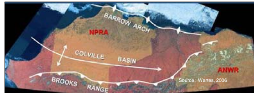
Figure 23 : Tectonic terranes in the Alaska North Slope region, showing the extent of Cretaceous and Tertiary foreland basin sediments in the Colville Basin. Sedimentary rocks in the Brooks Range are uplifted and deformed, thus not considered good targets for CO 2 storage.
