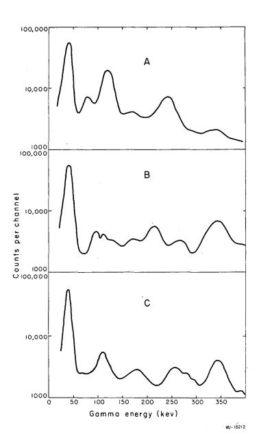
Fig. 1. Gamma spectra of terbium isotopes by alpha-particle bombardment of enriched europium isotopes. (A) 37-Mev alphas on  ${\tt Eu}^{153}$ , 3 x 3-inch NaI(Tl) detector; (B) 37-Mev alphas on  ${\tt Eu}^{151}$ , 3 x 3-inch detector; and (C) 48-Mev alphas on  ${\tt Eu}^{151}$ , 1.5 x 1-inch detector.
