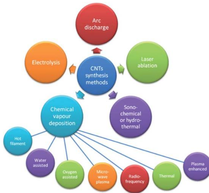
Figure 2.3 Currently used methods for Carbon Nanotube synthesis [37]
