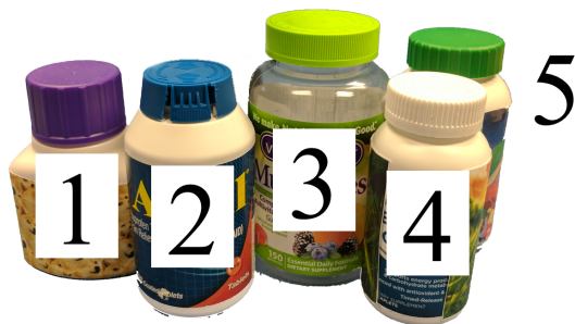
Figure 2.21: Bottles used in experiments with different safety mechanism: (1) push-and-twist , (2) pinch-and-twist , (3) push-and-twist , and (4) push-and-twist . (5) Bottle with no safety mechanism.
