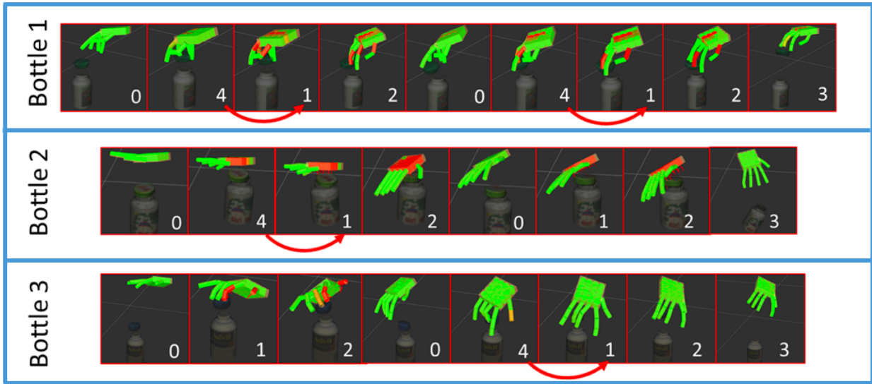
Figure 2.18: Key frames of opening various bottles with T-AOG. The numbers indicate the cluster labels and the red arrows indicate the merges triggered by the parsing of T-AOG.
